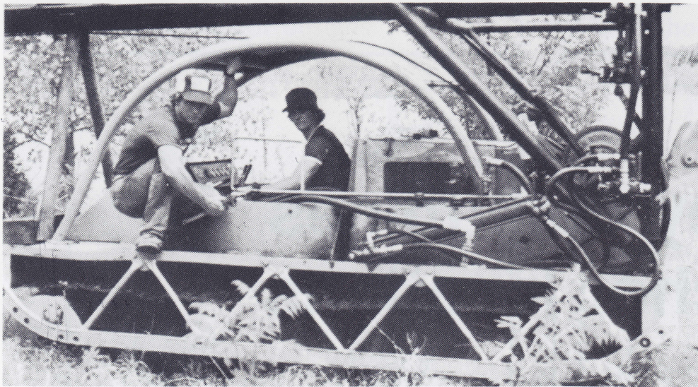
Dry land work. With boom retracted, the muskeg tractor crosses higher ground to make another test on auger anchors.
